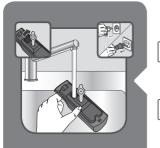
Fill the water tank with 100% water and repeat the operation until the water tank is completely empty in order to rinse the appliance.
